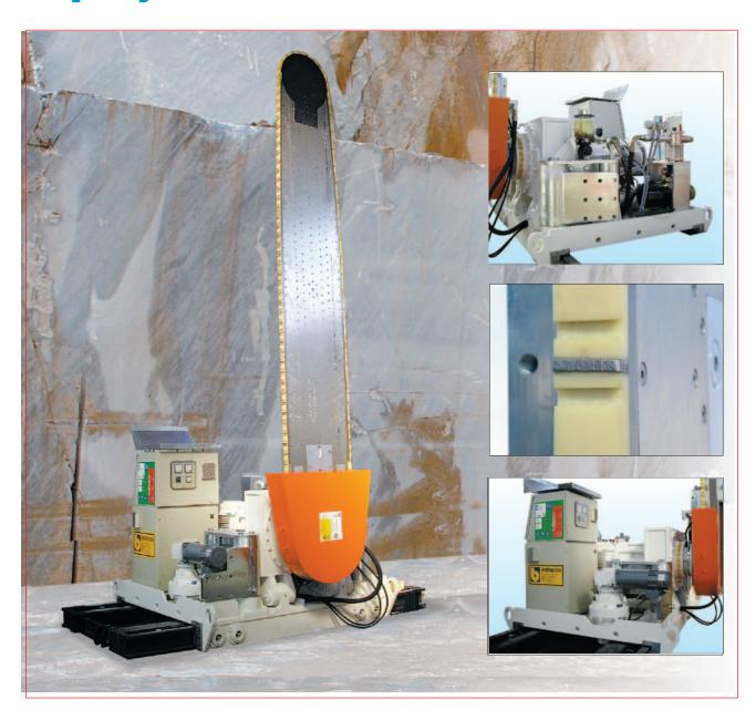
Diamond belt saw for vertical and horizontal cuts The cutting tool is a special plastic belt with sintered diamond segments that need NO grinding or
