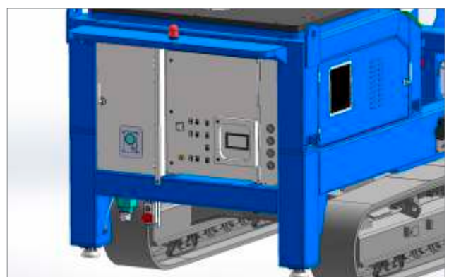
Quadro elettrico con pannello interfaccia operatore touchscreen Electric control panel with touch-screen
